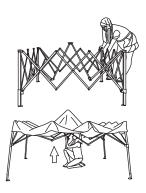
Lift one corner each time and walk backwards to expand the frame further. You may also walk into the gazebo and push up the gazebo under it to expand the frame as much as you can.
