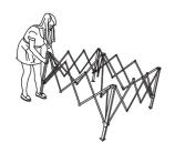
4. With all four corner locking released, lift and walk one corner of the frame towards the opposite corner to close the frame.
