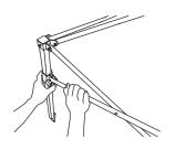
3. Release sliders at all four corners by pushing the red plastic button and gently push the sliders down to leave the locking position.
